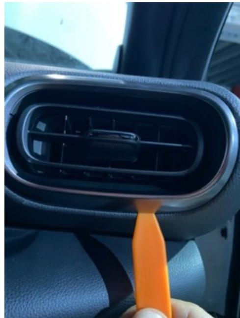
You can pull the whole vent from its place and put it on a table for further disassembling.
