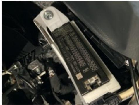
Find the Fuse "USB No.1" and remove it. Install the fuse adapter right in that place. The cover of the fuse box does not fit anymore. Please leave it in the car in case you need it in the future.
