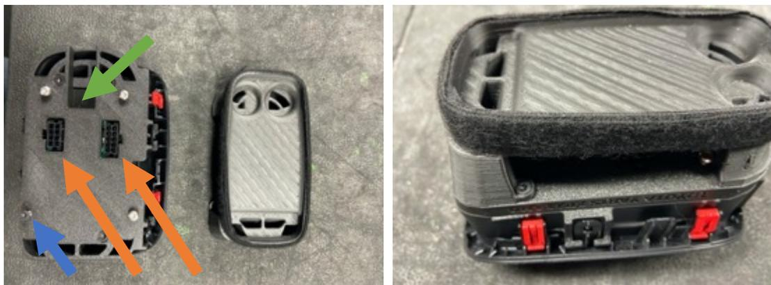
Remove the black screw from the back of the housing (blue arrow). Click in the air duct adapter and fix it with the black screw.
