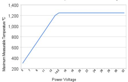
Maximum Measurable Temperature vs Power Voltage
